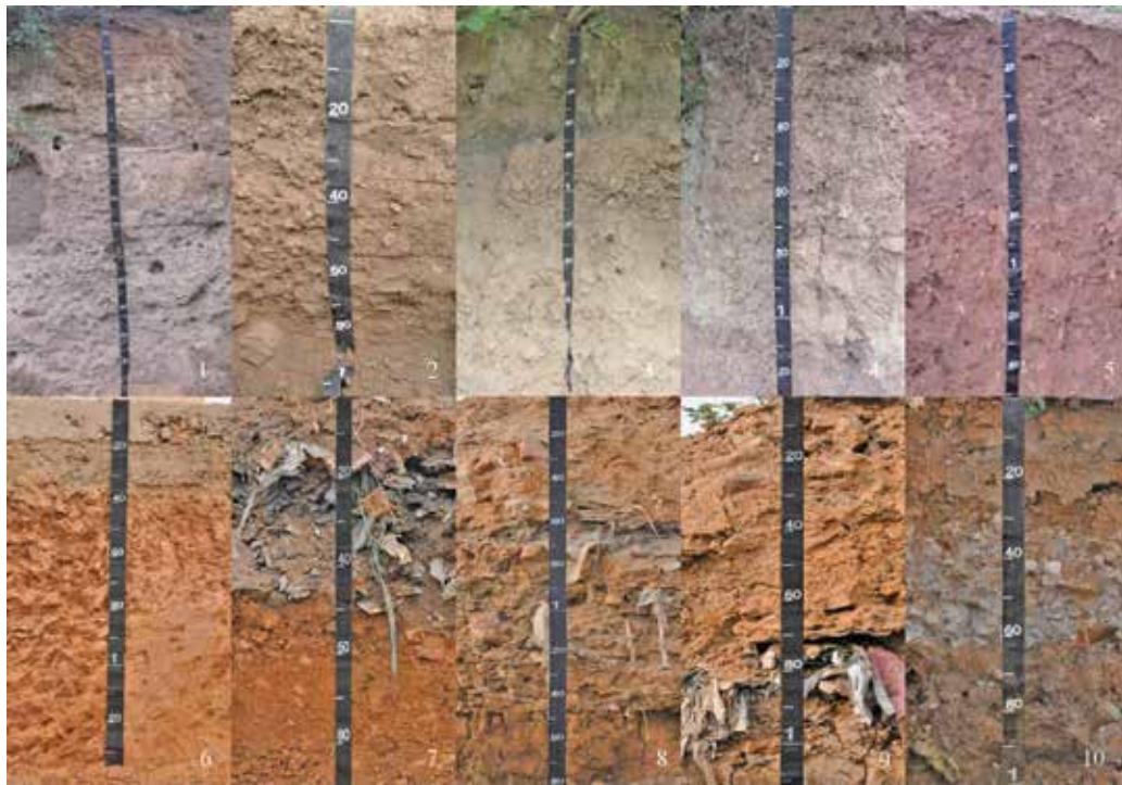
注：1.仰韶村遗址文化土壤剖面；2.汉魏洛阳城遗址文化土壤剖面；3.二里头遗址文化土壤剖面；4、5.无人工制品自然土壤剖面；6.道路封闭土壤剖面；7.生活垃圾堆积土壤剖面；8.废弃房屋土壤剖面；9.建筑垃圾堆积土壤剖面；10.废弃公路土壤剖面 Note: 1. Soil profile at the Yangshao village cultural relic site; 2. Soil profile at the HanWei Luoyang city cultural relic site; 3. Soil profile at the Erlitou cultural relic site; 4、5.Natural soil profile free of artifacts; 6. Soil profile of road closures; 7. Soil profile at a domestic waste dumping site; 8. Soil profile at a deserted building site; 9. Soil profile at a construction waste dumping site; 10. Soil profile at a deserted highway site
