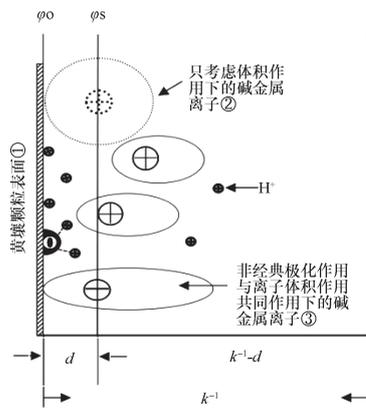
注：d为Stern层的厚度，κ<sup>-1</sup>为双电层的厚度，κ<sup>-1</sup>-d为扩散层厚度；φ<sub>0</sub>为表面电位；φ<sub>s</sub>为Stern电位 Note: d stands for thickness of the Stern layer; κ<sup>-1</sup> for the thickness of the double layer; κ<sup>-1</sup>-d for thickness of the diffusion layer; φ<sub>0</sub> and φ<sub>s</sub> for surface potential and Stern potential, respectively. ①Surface of yellow earth particles ②Alkali metal ion with volume effect ③Alkali metal ion with the volume effect and the non-classical polarization
