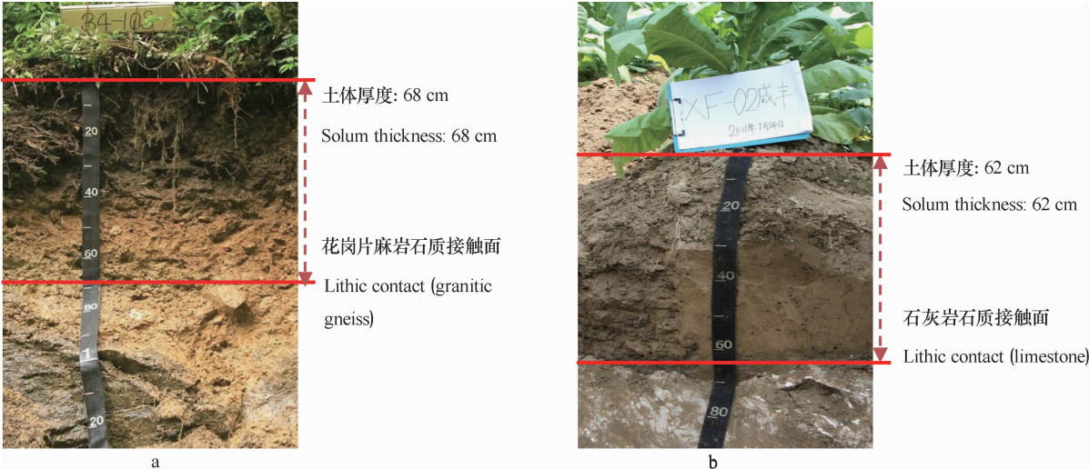
图 2 基于石质接触面的土体厚度划分 Fig. 2 Solum thickness partitioning based on lithic contact
