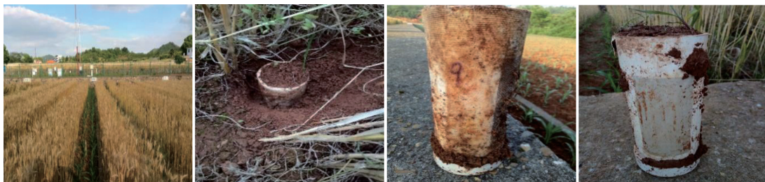
注: 从左到右依次为祁阳试验田、试验田埋入的柱子和试验完成后取出来的柱子 Note: The figure from left to right is the Qiyang experimental field, the column embedded in the experimental field, and the columns taken out after the test, respectively
