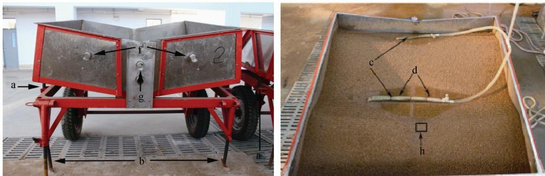
注：a. 垄向坡度调节螺旋；b. 坡面坡度调节螺旋；c. 供水管；d. 垄沟内调节水面的排水管；f. 上坡位置产流产沙收集口；g. 垄面下坡位置产流产沙收集口；h. 垄面最低处。Note: a. screw for adjusting row grade; b. screw for field slope adjustment; c. water supply pipe; d. drainage pipe for adjusting water level in furrow areas; f. outlet to export runoff and sediment from the upper area; g. outlet for collecting runoff and sediment from the downslope area; h. the lowest point at the ridge.
