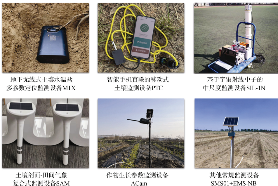
图2 基于传感器技术的农田土壤和作物信息监测设备 Fig. 2 Farmland soil and crop information monitoring equipment based on sensor technology
